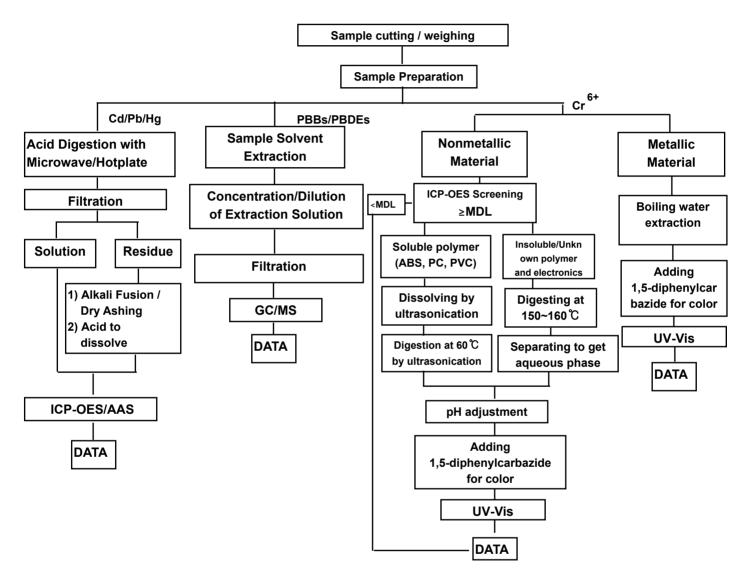
The samples were dissolved totally at the acid digestion step of the above flow chart for Cd,Pb,Hg Section Chief : Hwangsik Kim
